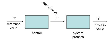
assumption: undisturbed operation ⇒ process value = reference value
