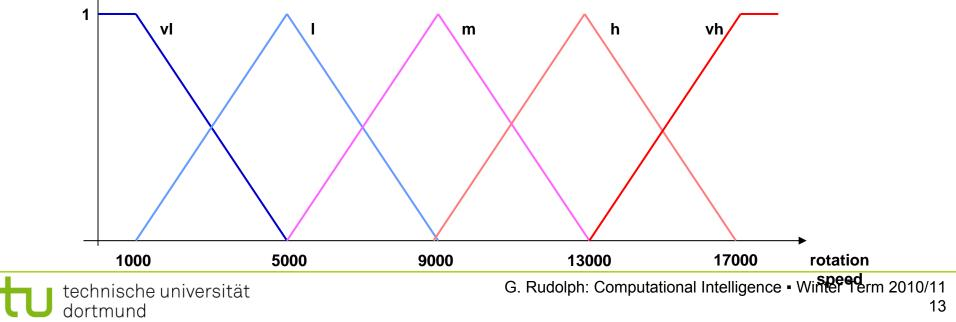
industrial drill machine  $\rightarrow$  control of cooling supply
