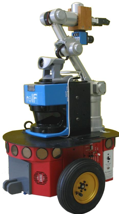
Abb. 1.1: Experimenteller Serviceroboter
