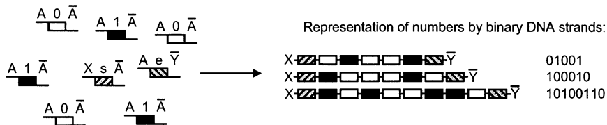
Fig. 1. Assembly of DNA binary strands. All binary strands are of the form s\{0|1\}e (EBNF after ISO14977), yielded by concatenation of two terminators s (start) and e (end) and an arbitrary number of DNA bits in between. Concatenation was performed by annealing and ligation. Terminators and DNA bits are made of annealed complementary oligonucleotides having sticky ends ( A , \bar{A} , X , \bar{Y} ) for concatenation on both sides. The sticky end A ( \bar{A} ) works as a variable for correct concatenation of bits and terminators, whereas X and \bar{Y} are sticky ends required for subsequent cloning. Bits and terminators were represented by unique double stranded DNA sequences which overlap in 26 bp and contain sticky ends of 4 nucleotides length. Bit strands containing up to 32 bits were yielded from the subsequent ligation reaction (Data not shown, see Section 9).
